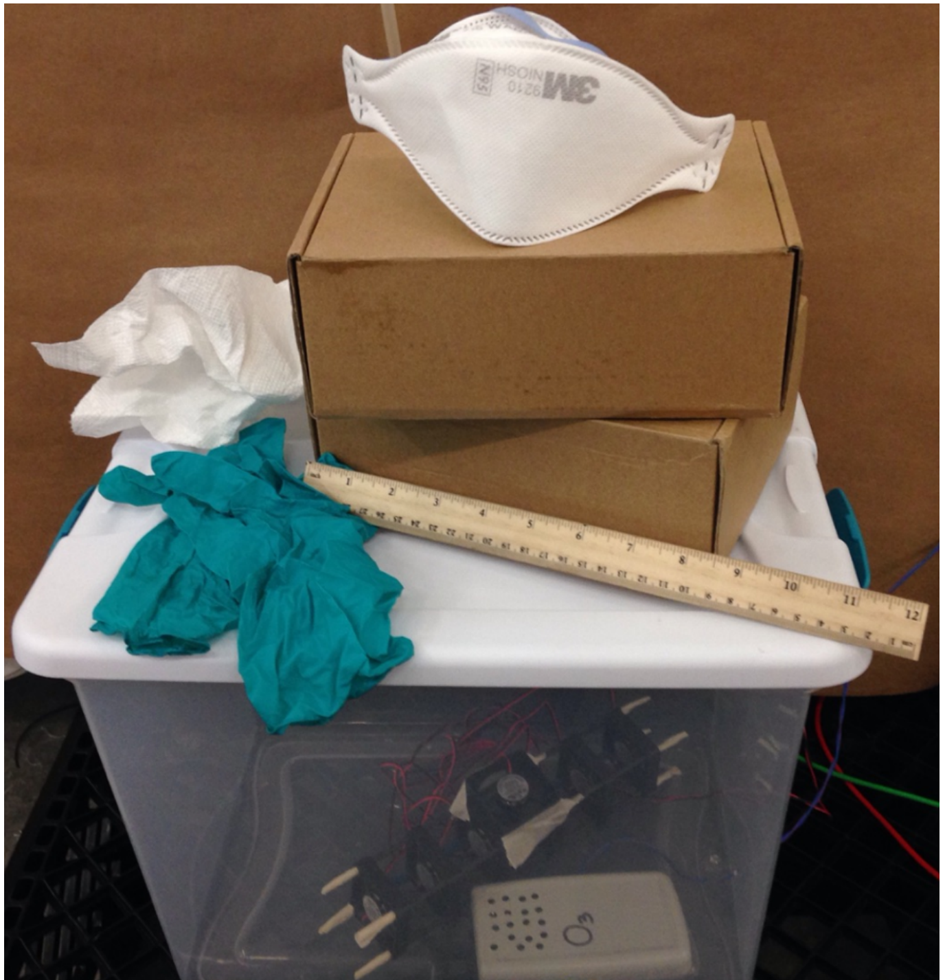
Figure 2. Ozone quenching effect of the materials being disinfected. For one experiment, materials were added into the box for a disinfection cycle to measure the effect of these materials on ozone concentration (quenching).
