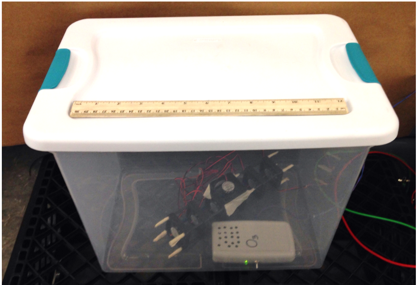
Figure 1. Test box (24-liter size) showing the box fan array and ozone sensor located in the bottom of the box. A 12-inch ruler is included for scale.
